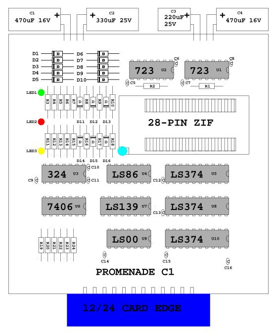
The ZENER diodes (1N4739 and 1N4740 rated at 1W) get hot during operation. I have replaced the diodes on my programmer with a higher rated diode (1N5346B and 1N5347B rated at 5W). Also raise them up off the board as much as possible, the leads act as heat sinks.
